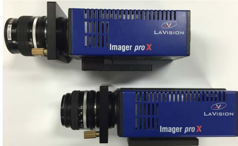
Figure 3.9: Imager ProX CCD cameras used for PIV measurements.
